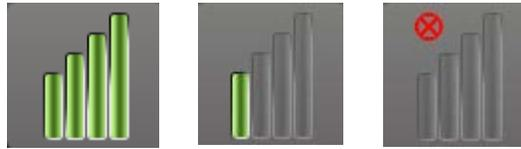
Figure 7: Link Quality Indicator (Excellent, Poor, No Link)
