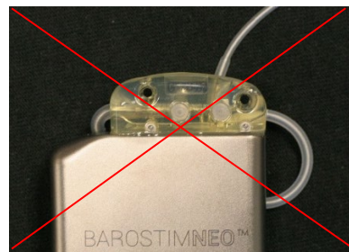
Incorrect Placement of Lead Behind IPG
