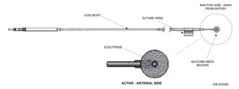
Figure 3: Carotid Sinus Lead
