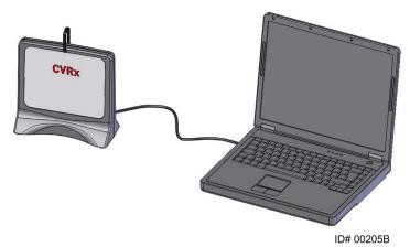
Figure 6: Programmer System Model 9010
